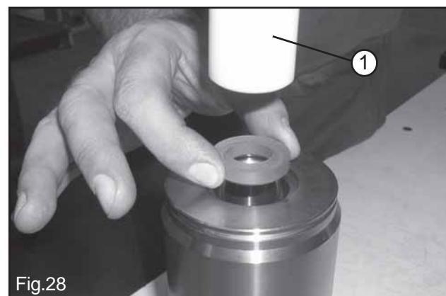
Each pressure packing set component should fit tight in the cylinders because of a little interference designed in the ext. diameter. A pin of adequate dimensions (1, Fig.28) helps in guiding each component straight and aligned all the way down in the cylinder.
