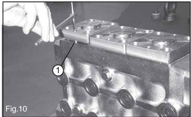
Tighten the two grub screws 1, Fig.10 of each valve cover till the complete valve unit moves upwards enough to allow easy extraction.
