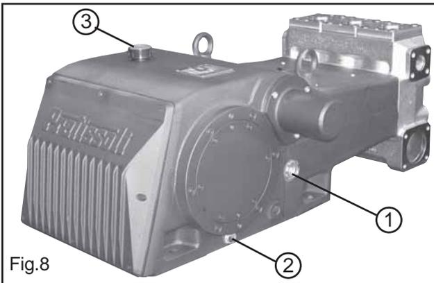
If necessary, top up from the oil plug 3, Fig.8.
