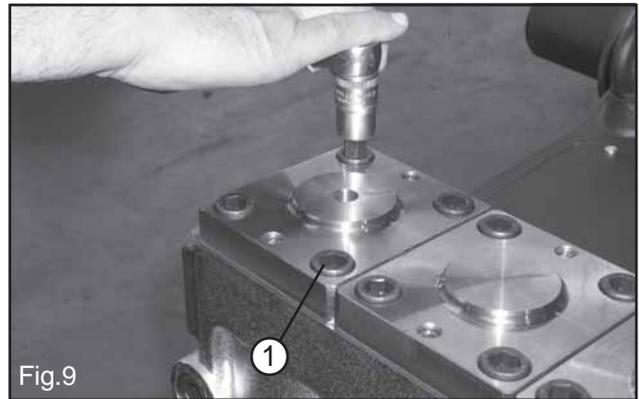
Loose and remove the valve cover screws 1, Fig.9.
